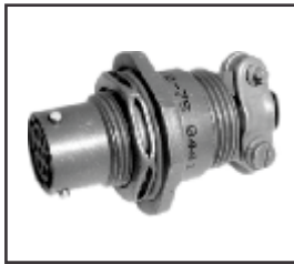
62 IN - 14F Single hole mounting with grommet and grommet nut with integral strain relief clamp has panel 'O' ring seal
